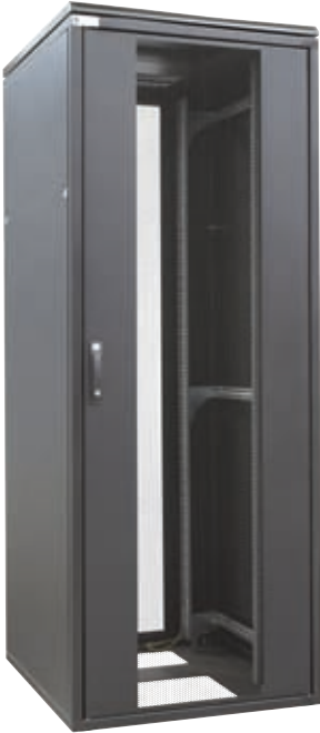
Cabinet SZB SE 42 U, 800x1000 mm, colour: RAL 9005, set on levelling feet, door with perforation type C, two pairs of mounting profiles in 19" spacing Catalogue no. WZ-SZBSE-005-5711-11-0000-2-161
